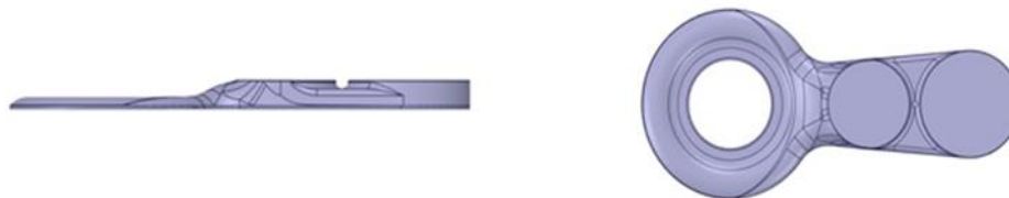
Figure 6: Volume of combustion chamber when piston at TDC
